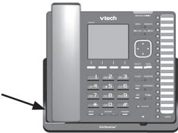
4. Lift the deskset base to the desired angle. There are three pairs of grooves designed to hold the phone at different angles for optimum visibility.
